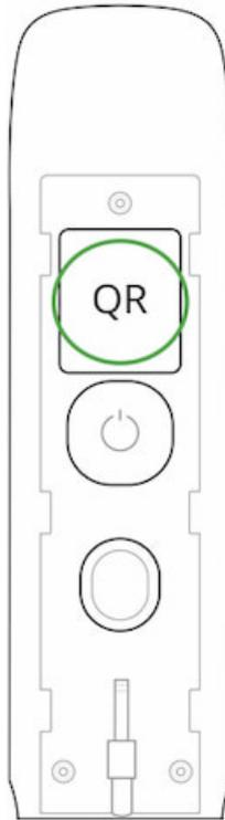
3. Turn on the detector by holding its power button for 3 seconds.
