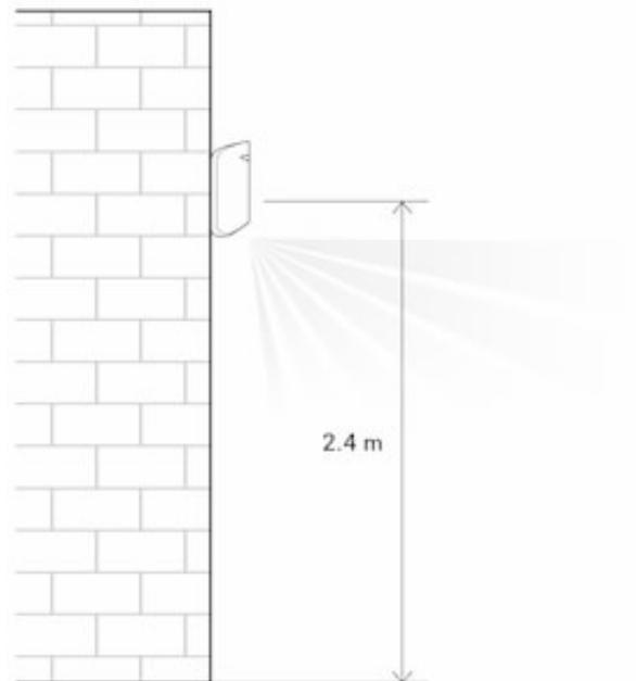
Installing the detector at any other height will narrow the detection zone, affecting the quality of motion detection.
